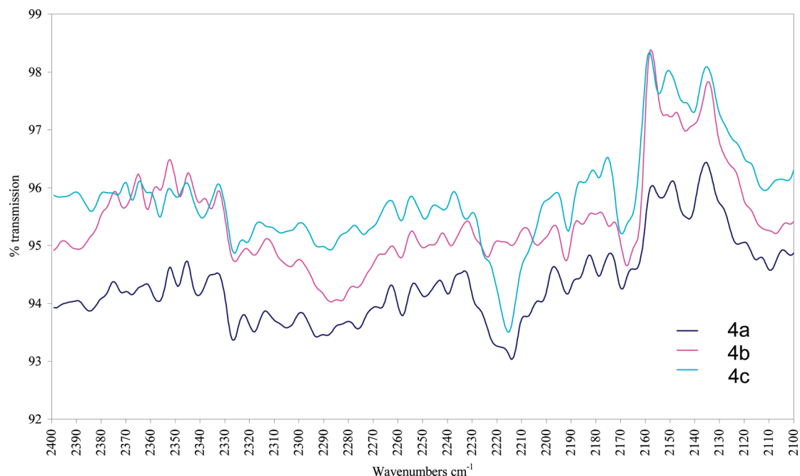
Figure 13. Partial FT-IR (ATR) spectra of newly reported dicyanate homopolymers 4a , 4b , and 4c cured at 180 and 230 °C/h (showing expansion of cyanate region).
